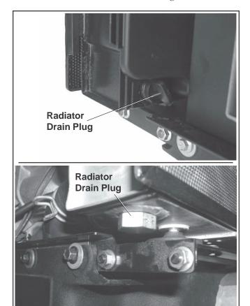
Figure 11. Radiator Drain Plug Location.
